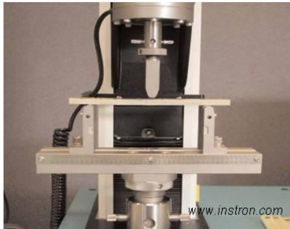
Figure 2.9.2. Example of three-point bending test
