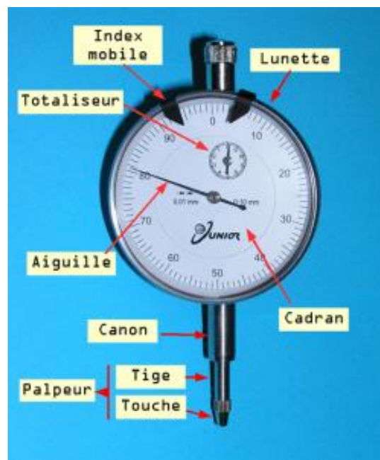
Figure 2.4.8. Schematic view of a comparator
