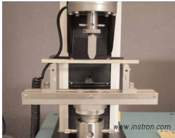
Figure 2.9.2. Example of three-point bending test
