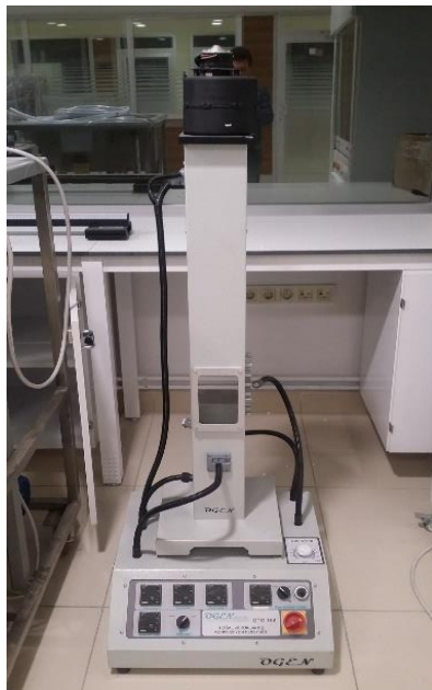
Figure 2.8.2. Convection experiment unit
