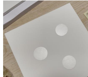
Fig. 5 Macroscopic appearance of E, F, and G YSZ electrolyte samples. Surface integrity is maintained with increasing pressure.
