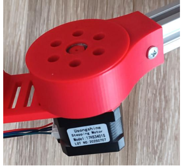
Fig. 3 Cycloidal reducer connection to NEMA 17 stepper motor
